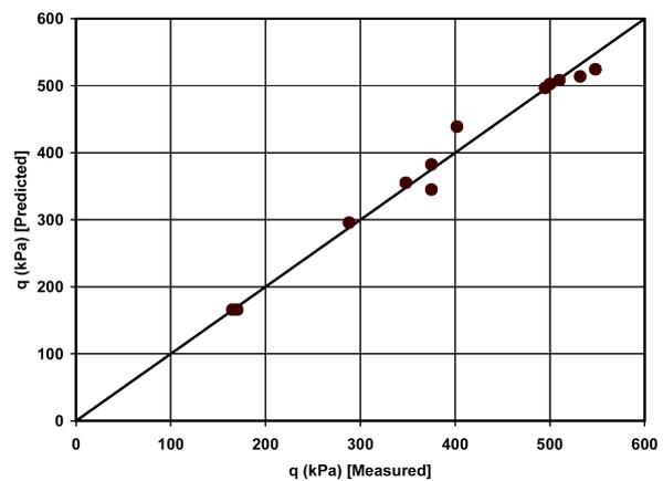
**Fig. 12.** Comparison of measured and estimated values of deviator stress, q, based on hyperbolic tangent function
