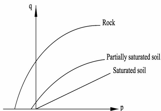
**Fig. 1.** Mechanical behaviour transition of soils in saturated to fully dry states
