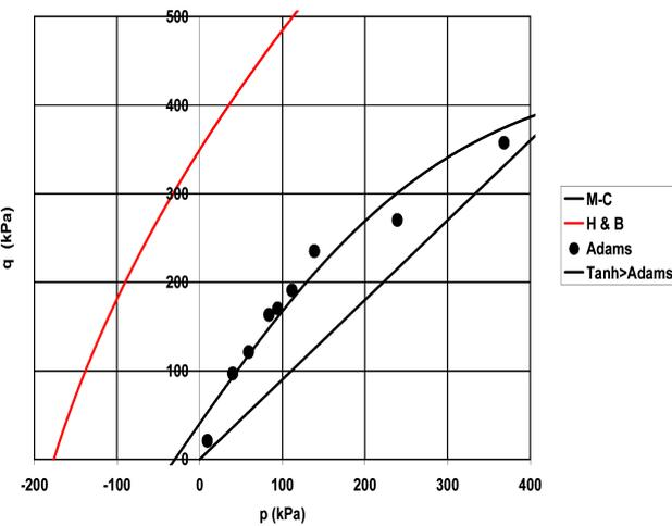
**Fig. 7.** Curve fitting for Adams and Wulfsohn (1998) data by a hyperbolic tangent function
