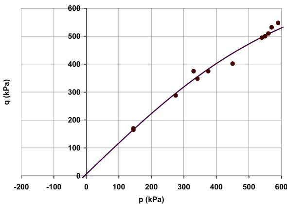
**Fig. 11.** Hyperbolic tangent function obtained from experimental results
