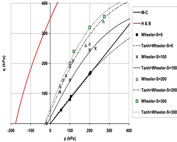
**Fig. 5.** Curve fitting for Wheeler and Sivakumar (1995) data by a hyperbolic tangent function
