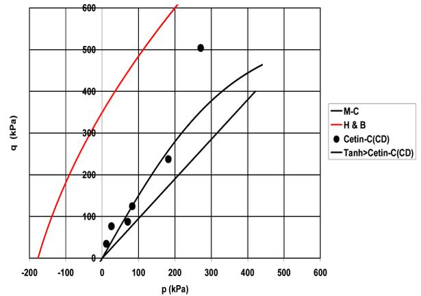
**Fig. 10.** Curve fitting of Cetin (1999) data for soil C as a hyperbolic tangent function
