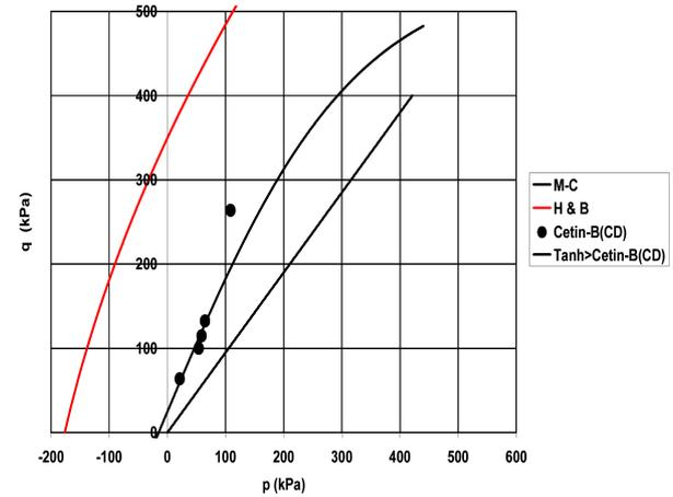
**Fig. 9.** Curve fitting of Cetin (1999) data for soil B as a hyperbolic tangent function
