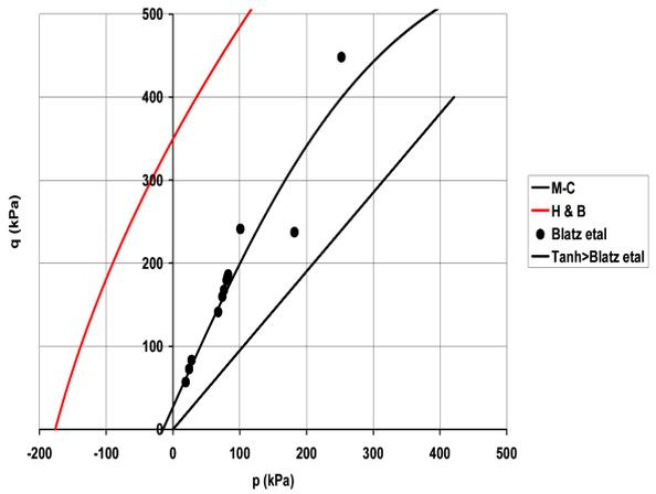
**Fig. 6.** Curve fitting for Blatz et al. (2002) data by a hyperbolic tangent function
